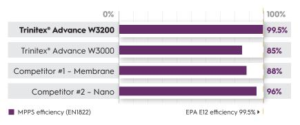
**Trinitex Advance W3200 is a true E12** according to EN1822, reaching >99.5% MPPS efficiency.
